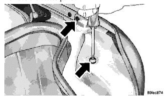
2. Twist sockets counter-clockwise to pull out bulbs. Replace tail, tail/stop, or marker lamp bulb.
